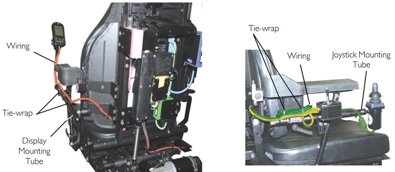
**FIGURE 2.6** Recommended Wire Routing and Securing Points - Contoura Back
