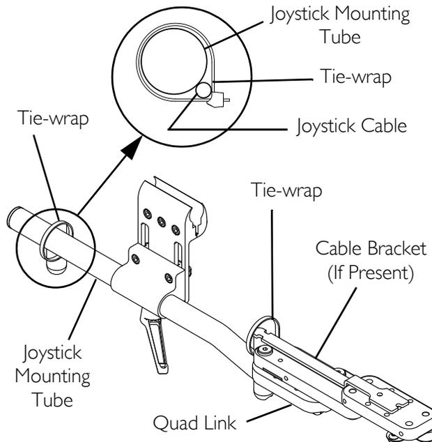
**i** The use of a cable bracket with a quadlink joystick mount is strongly recommended to reduce stress on the joystick cable.
