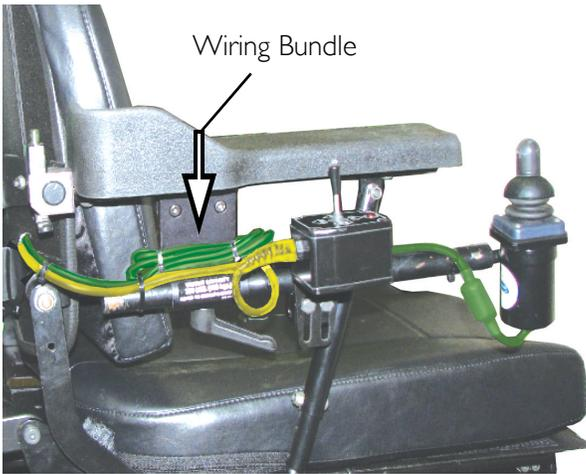
**i** Examples of excess wiring gathered into bundles before being secured to the wheelchair. Images are examples of wire bundling ONLY. Location of electronic components and wiring may vary from wheelchair to wheelchair according to wheelchair model, manufacturing date, options or accessories. ALL WIRING, CONNECTOR STACK, AND CONTROL BOXES **MUST** BE PROPERLY SECURED TO THE WHEELCHAIR BEFORE USE.
