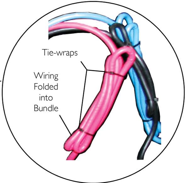
FIGURE 2.2 Bundling the Wiring
