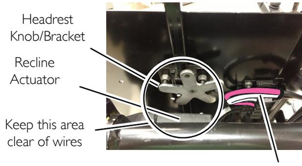
**i** Refer to Bundling the Wiring on page 10 for correct routing of excess wires.
